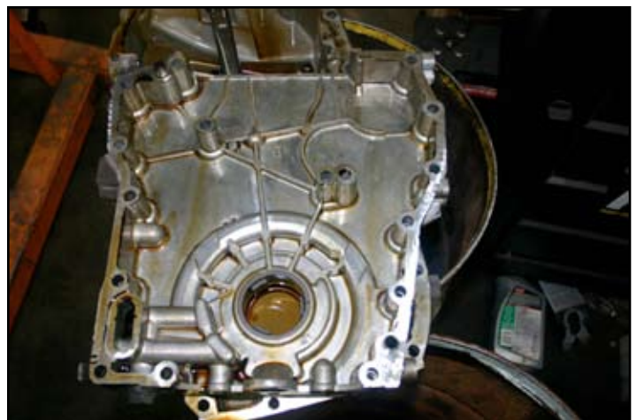
Internal side of the out-of-spec oil pump. There is no evidence of oil sludge or varnish deposits. All photographs by the author.
