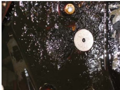
Oil pan showing debris in H.C. Thing's Aero. It is bad but not nearly as bad as the silver rapper!
